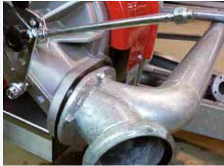
Transparent painting for boosting the protection of galvanized parts.
