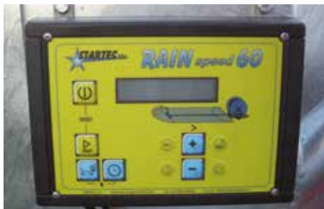
Rain Speed 60 digital metre counter for measuring the rewinding speed.
