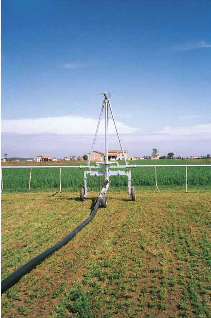
Steel boom for distributing sludge from 28 metres with descent
