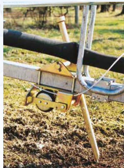
Device for locking trolley to the ground with pickaxe (for models with rear hose unwinding).
