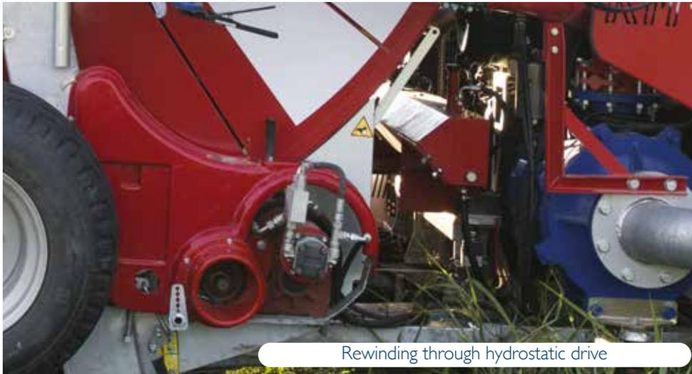
Rewinding through hydrostatic drive
