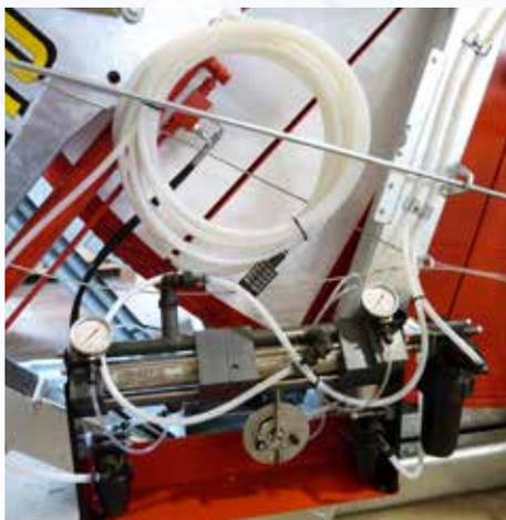
Dosing pump for sewage irrigation with liquid fertiliser.
