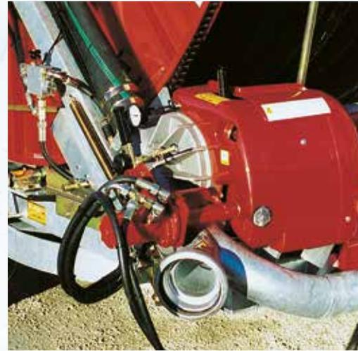
PE hose rewind through hydraulic motor on PTO, speed adjusting valve, limit switch spool valve and quick coupling torque to tractor:
