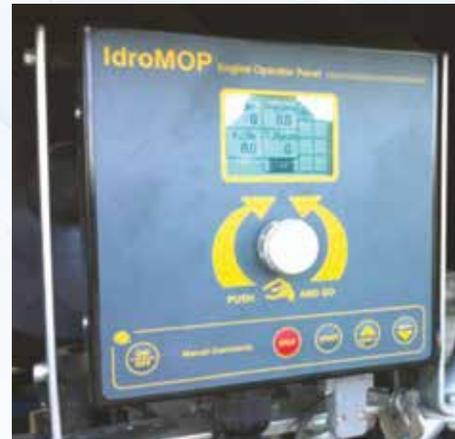
IDROMOP programmer for jointly controlling the irrigation machine + diesel engine on the XJM models.
