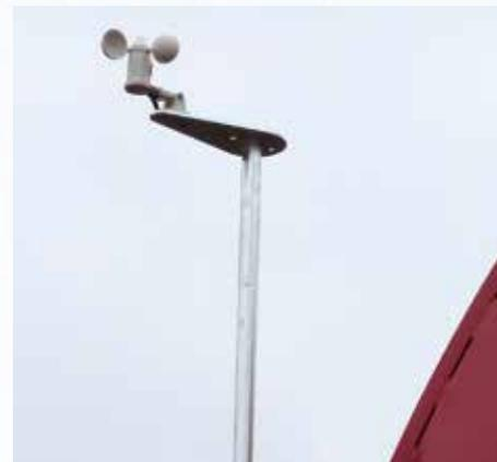
Anemometer for Rain Master 2.6
