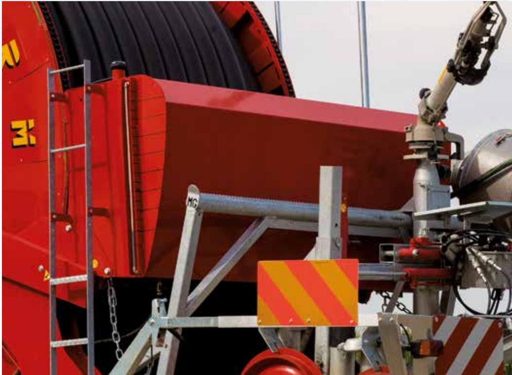
All the XJM models are fitted with a great-capacity fuel tank with a vertical development. This makes it impervious to the machine tilt variations. It is not incorporated into the frame, and it is positioned between diesel engine and reel, or in the rear in the MAGNUM Xjm models.
